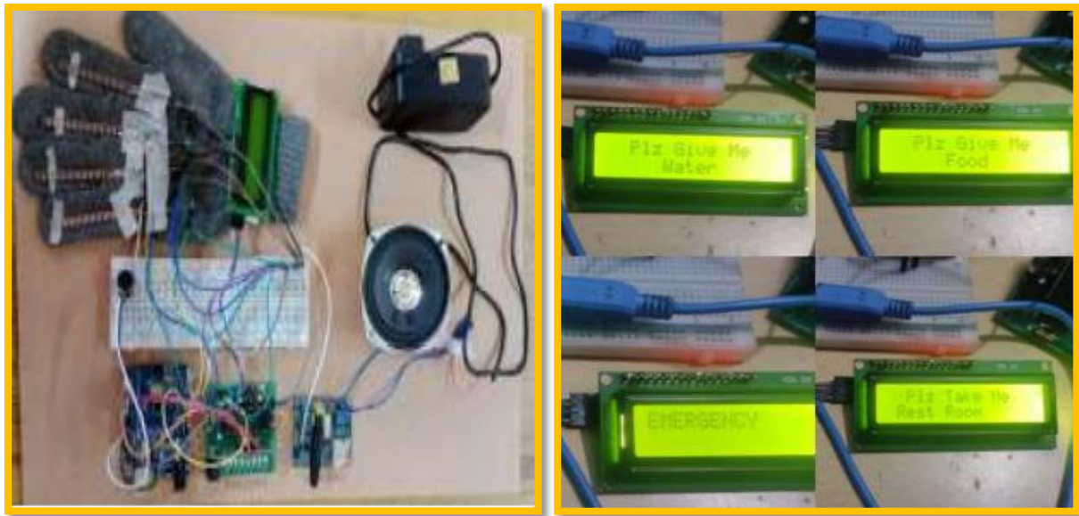
Figure 7.2 Working model with messages displayed on LCD
